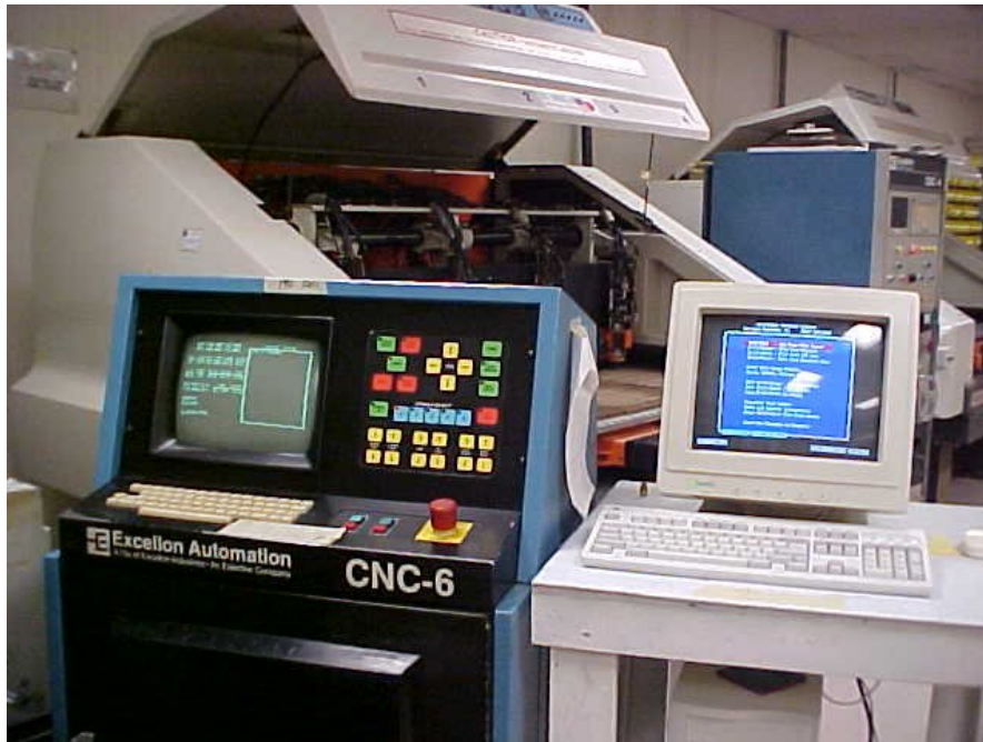
Figure 2. Excellon CNC-6 with computer connected via paper tape reader port
