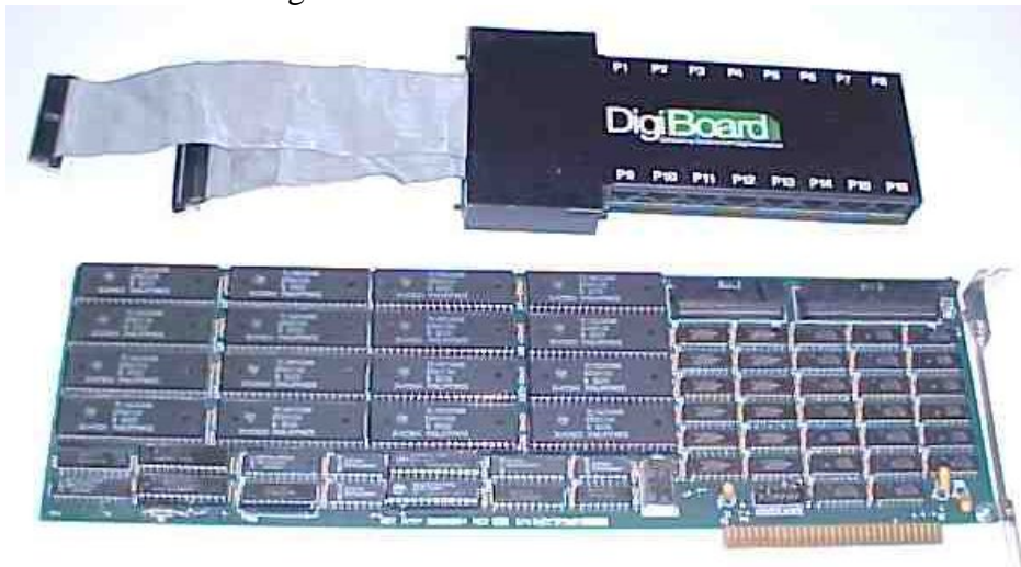
Figure 17. 16 Port Digiboard use in original Excellon Miniserver
