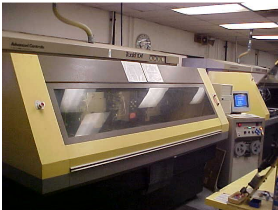
Figure 3. TruDril 104 with computer connected via paper tape reader port
